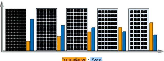
Module's power output increases along with the decrease of the light transmittance.
